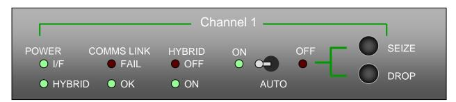
When in Auto mode, an incoming call will be answered with a blip of 2 tones being sent down the line. The tones are an indication to the caller to enter the Direct Dial DTMF tones, if required, to call an individual panel within the Telephone group. This feature is only available when the TIC card is installed. This is set up in the configuration software.
